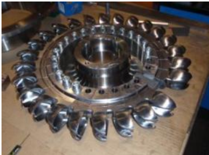
Photo 31. Achievement of a Pelton runner with mounted buckets (St Jean SHP plant, Switzerland, set in a drinking water network, H = 373 m, Q = 34 l/s, P=102 kW, 2009).
