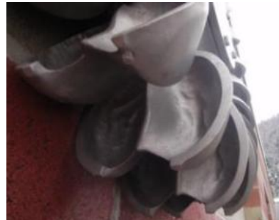
Photo 32. Pelton bucket worn out by sand particles (case study Le Châble-Profray).
