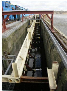
Fig. 11. Frame with fixed the current meters for traversing the hydrometric (measuring) section (author's application).
