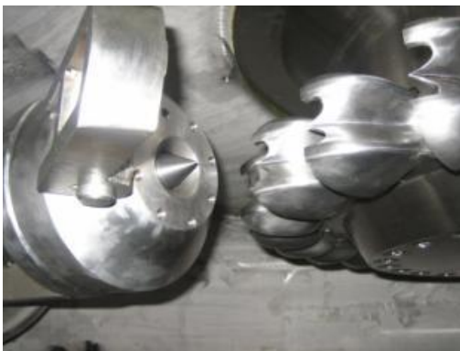
Photo 37. A deflector before the commissioning (case study le Châble Profray).
