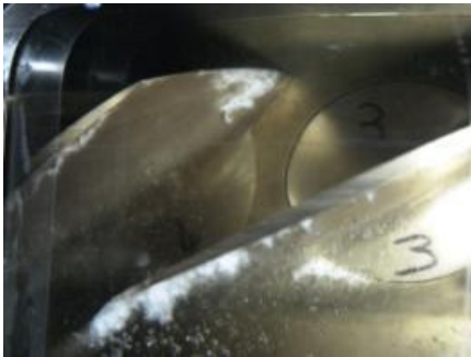
Photo 35. Cavitation on blades for a Kaplan runner.
